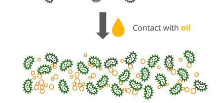
Bacteria proliferate inside the cable, degrading the **oil** and producing **biosurfactants**.
